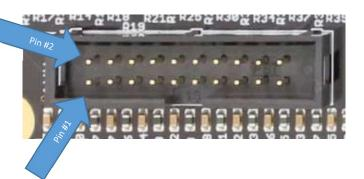
Each input has a pull-down, this means that when no signal is connector the board will see a 'low' signal. Connecting an input to 24V will cause the board to detect an 'high' signal.
