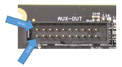
This output can directly be used, for example, to switch a relay. If a logic signal is needed a pull-up resistor is required.
