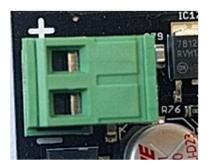
**Warning:** Check the polarity of the power, damage to the board may occur if the polarity is reversed.
